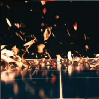
Wind Load Test IEC61215 TUV Standard
