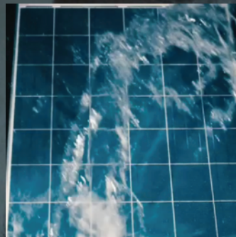
Waterproof Test IEC61730 TUV Standard
