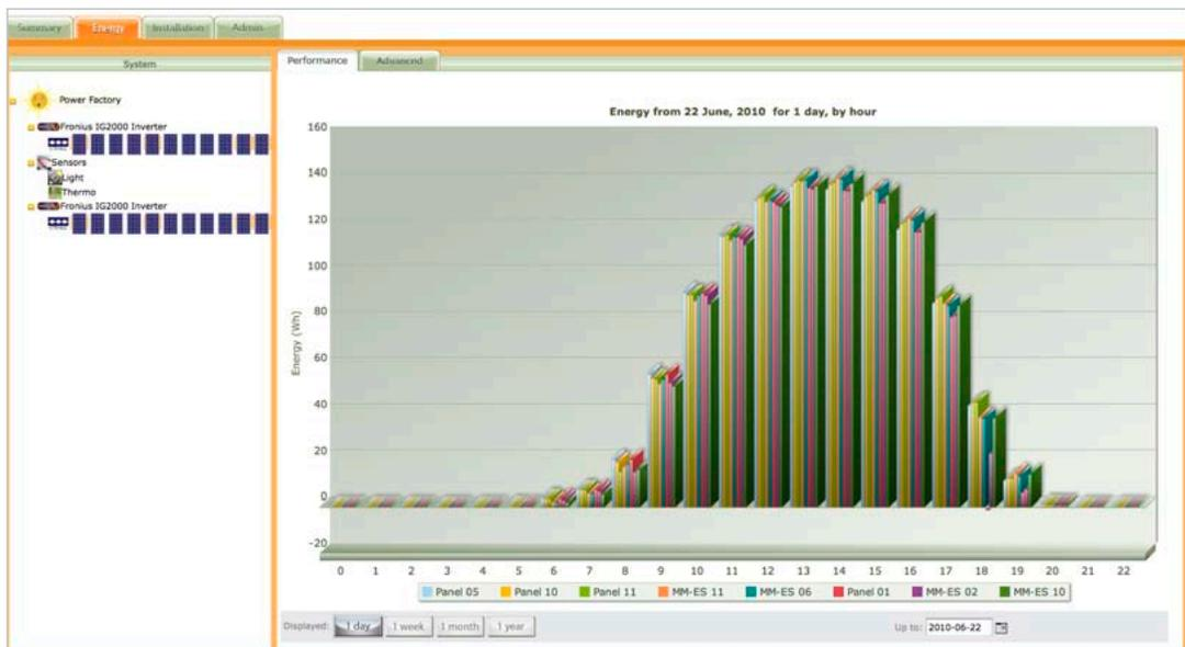
By clicking on the Advanced sub-tab, choose to compare objects by power, temperature, voltage and a number of other variables. In the bottom right corner, click the Download button to export the raw data to a .CSV file format, or choose Open Graph button to view the data in a Java based graphing tool.
