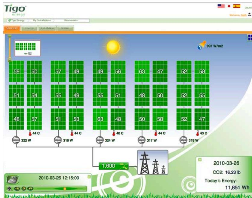
If the installer has included an optional light sensor, the sun intensity (irradiance, measured in Watts per square meter - W/m<sup>2</sup>) is indicated in the upper right hand corner above the modules. Similarly, if the system is equipped with temperature sensors, the ambient or module temperature (depending on the placement of the sensor) will be displayed next to the small thermometer icon.
